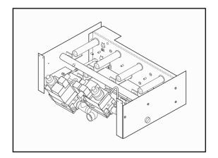
6. Before returning the burner group to its place, check that the separation between the ignition electrode and the far burner is between 2 and 3 mm.
