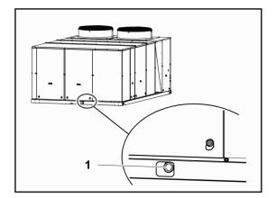
Install a drain trap on the exhaust outlet of the unit. The drain trap should be fitted with an access hatch -1- for easier draining and cleaning where required.
