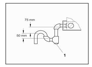
Lay the condensate drain pipe from the female connection on the bottom of the unit to a nearby drain.
