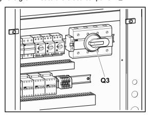
To correct the phase sequence, change the position of two of the three unit power cables on the input terminals.
