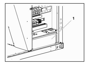
Pull the cables through the gland at the base of the unit. -1- and -5-.
